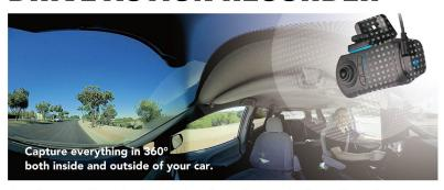
The DC5000A offers viewing angles of 360 degrees horizontally and 360 degrees vertically. d'Action's unique "Dual-recording" technology automatically crops the front facing footage to record it separately in higher definition (approximately 2.0 megapixels).
