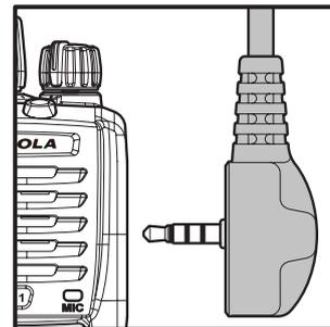
*Note 1): Save the original plastic cap and its mounting screws. They should be reinstalled when not using the Speaker/Microphone.*
