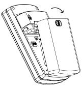
Install the three D batteries in the configuration illustrated to the right. Replace the battery sled, and slide the battery sled latch to the **CLOSED** position.
